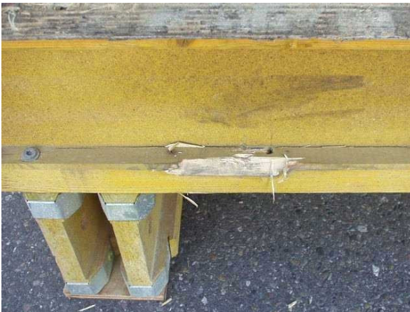
Photo 15 Permissible splintered edge
