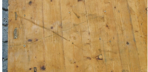
Photo 4 Permissible surface scratching
