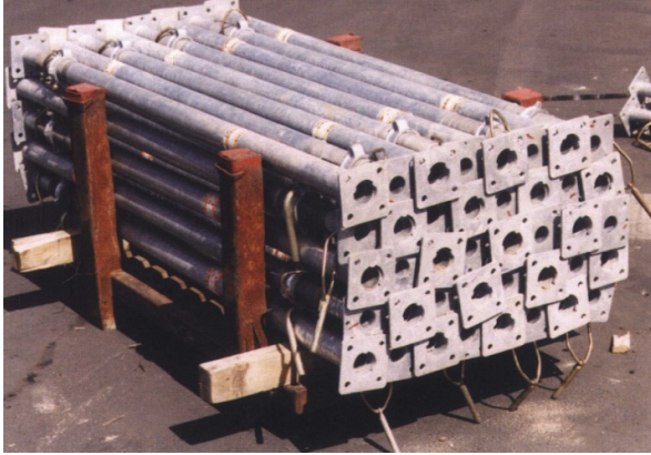
Photo 10 Used props, required cleaning condition
