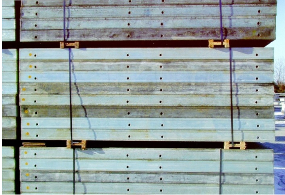
Photo 3: Example of required cleaning condition of the contact areas
